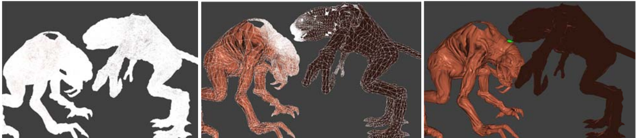
Figure 1: 200M polygons in wireframe (left), tessellated polygons in potential collision areas(center), collided polygons in green (right)
